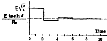
FIG. 85. Time variation of sending-end current on the open distortionless line of figure 82. Unity on the time scale is equal to the time required for the wave to travel the length of the line.
